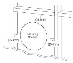
2. Determine the correct speaker location and use the template included with the speaker to mark the ceiling material.
