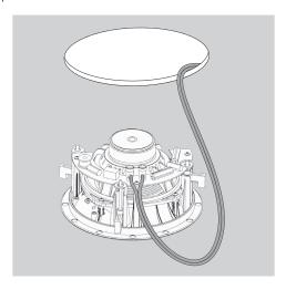
Attach the speaker's seismic tab to a support line, as per local safety regulations.
