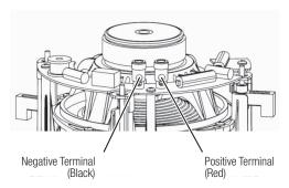
Press down on the post to open the hole; insert the bare end of the wire into the hole and release the post to secure the wire.
